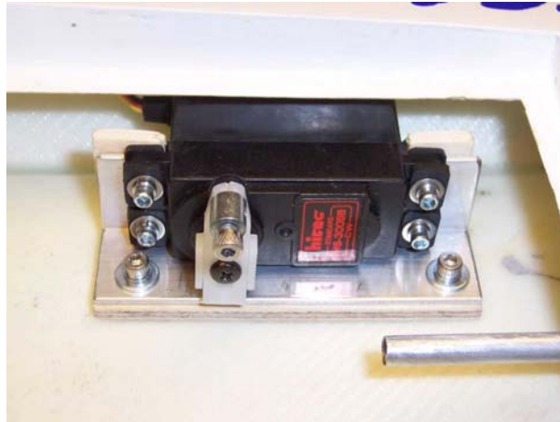
Photo 8: The completed servo mount installed in a hydroplane hull
