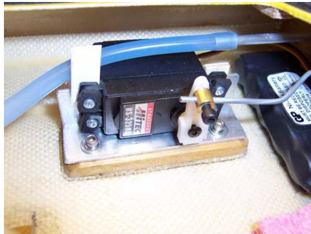
Photo 9: The completed servo mount installed in a mono hull
