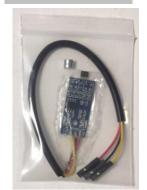
**Magnetic RPM sensor:** Stick the magnet on the motor's shaft, fix the sensor near the magnet, the sensor and magnet can not over 4mm, the green light illuminate means the sensor is working, if the green light off, try to change the magnet to the other side up or let the sensor nearer to the magnet until see the green light is illuminated.
